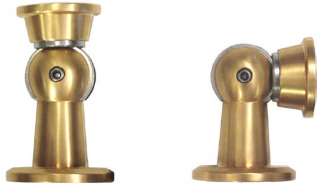
#34.MDHH Magnetic door holder Picture finish: Satin gold Wall or floor or ceiling mounted; For medium weight doors distance: 75.5 mm - 3"high . Brass base material, except for magnet Cup in receiver part galvanized steel.
